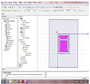
Fig. 2 Designed H-shape microstrip patch antenna
